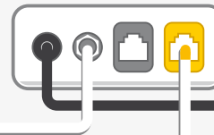
NBN™ Connection Box Connects to your modem via Ethernet to the WAN Port
