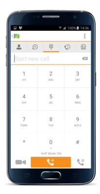
The *Dial Pad* tab displays a dial pad and a text field used to enter numbers. The dial pad is one of the options used to make audio calls. There are buttons below the dial pad: Call and Dial pad menu that are configurable by the service provider. The top text field also has a delete button that, when pressed, deletes one character at a time.
