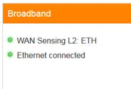
The **Broadband** card displays the status of the DSL or Ethernet WAN connection.
