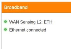
The **Broadband** card displays the status of the DSL or Ethernet WAN connection.
