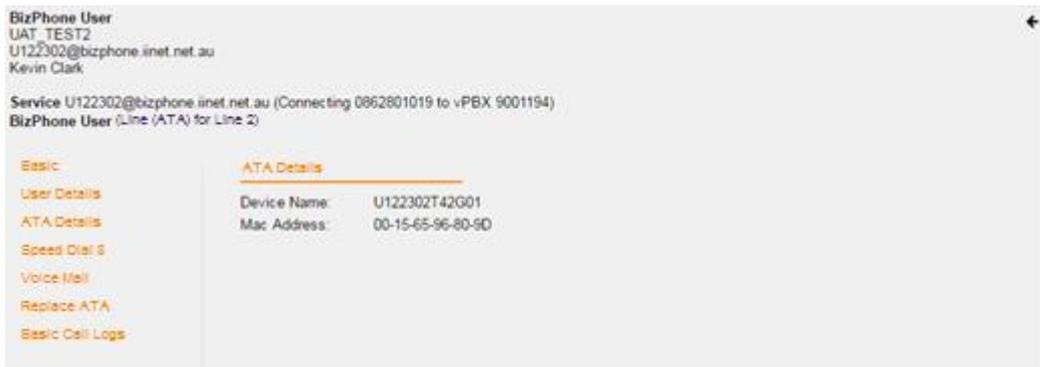
Note: The Handset/ATA Details go hand-in-hand with the Replace Handset/Replace ATA feature. If you replace your handset/ATA with a new or replacement handset/ATA, the new or replacement handset/ATA’s details (Device name and MAC Address) will be displayed in this page.
